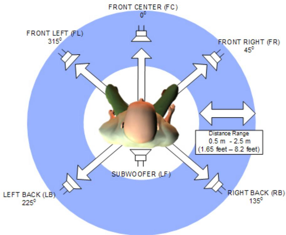
NOTE: The subwoofer may be placed in locations other than that indicated in this figure. Due to the potential for interactions with room acoustics and specific hearing instrument features, dispensers are advised to verify that their desired subwoofer location is acceptable to the manufacturers with whom they will be working.
