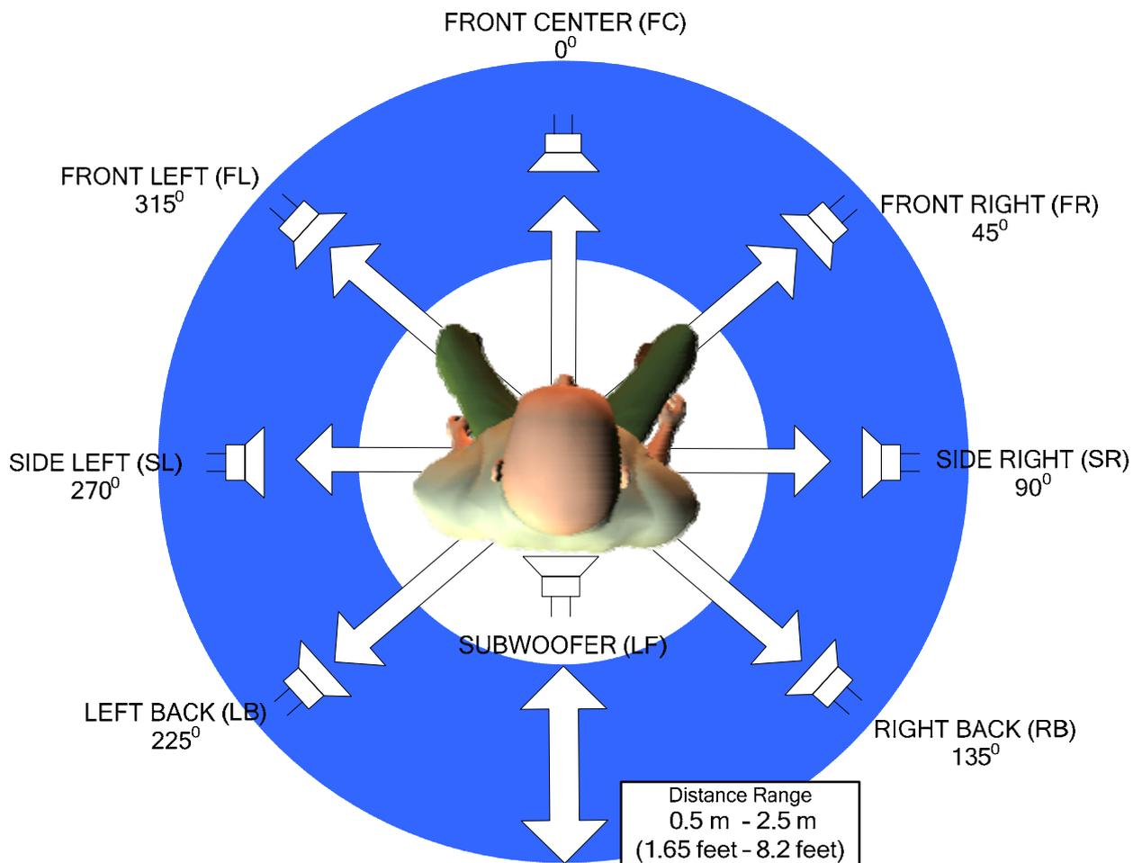
NOTE: The subwoofer may be placed in locations other than that indicated in this figure. Due to the potential for interactions with room acoustics and specific hearing instrument features, dispensers are advised to verify that their desired subwoofer location is acceptable to the manufacturers with whom they will be working.
